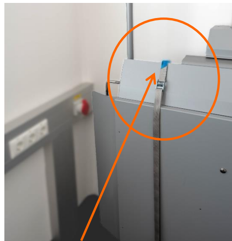
When a front mounted access ramp is fitted, pass the belt over the top edge of the ramp.
